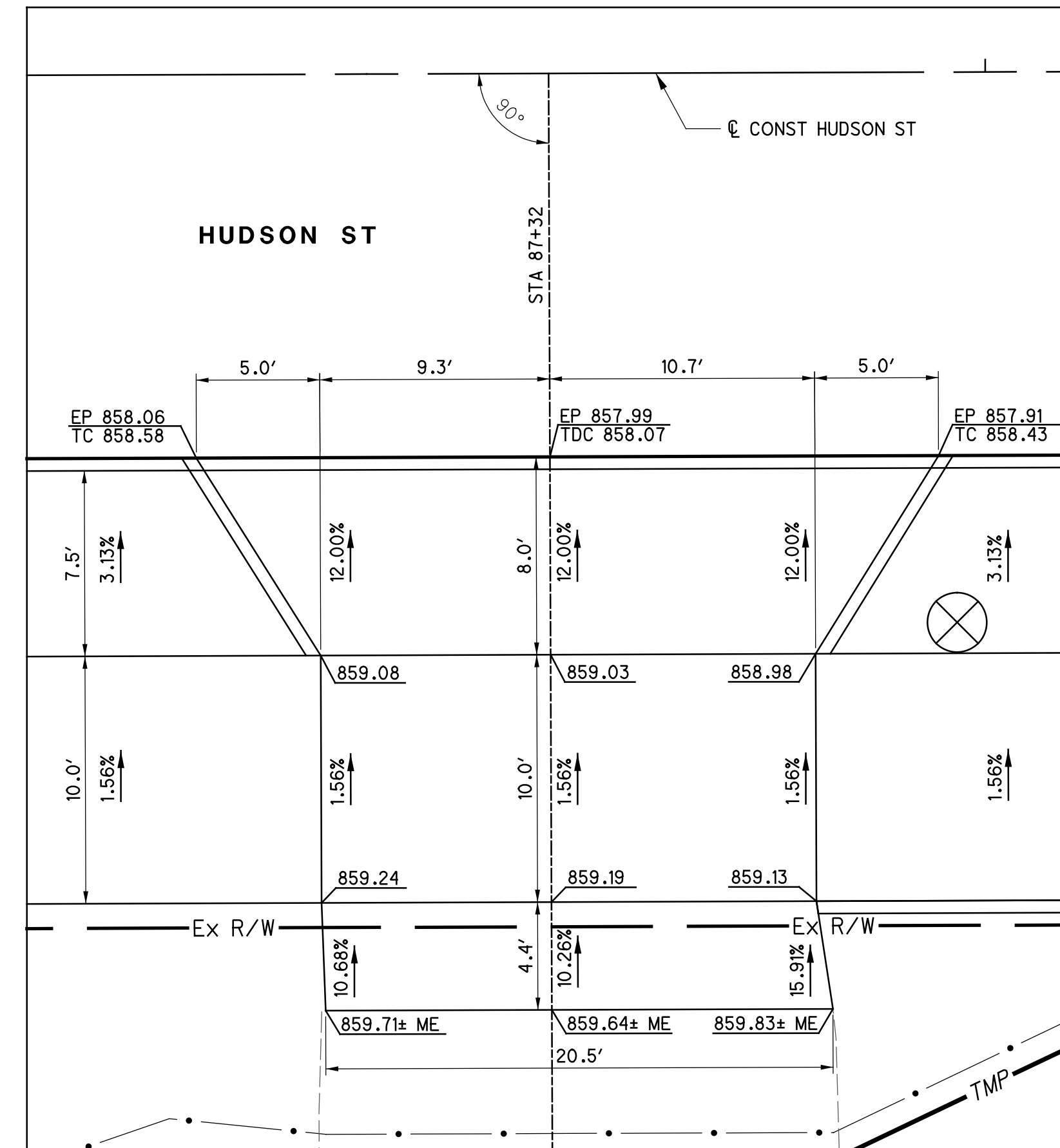
DRIVE DETAIL AT HUDSON ST STA 87+32 RT
