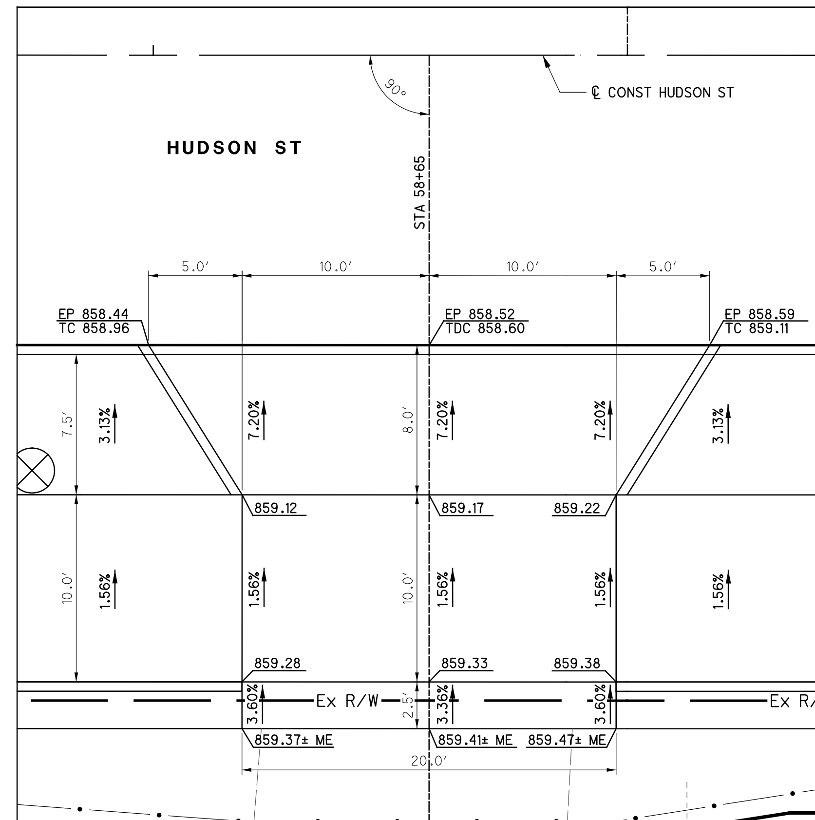
DRIVE DETAIL AT HUDSON ST STA 58+65 RT
